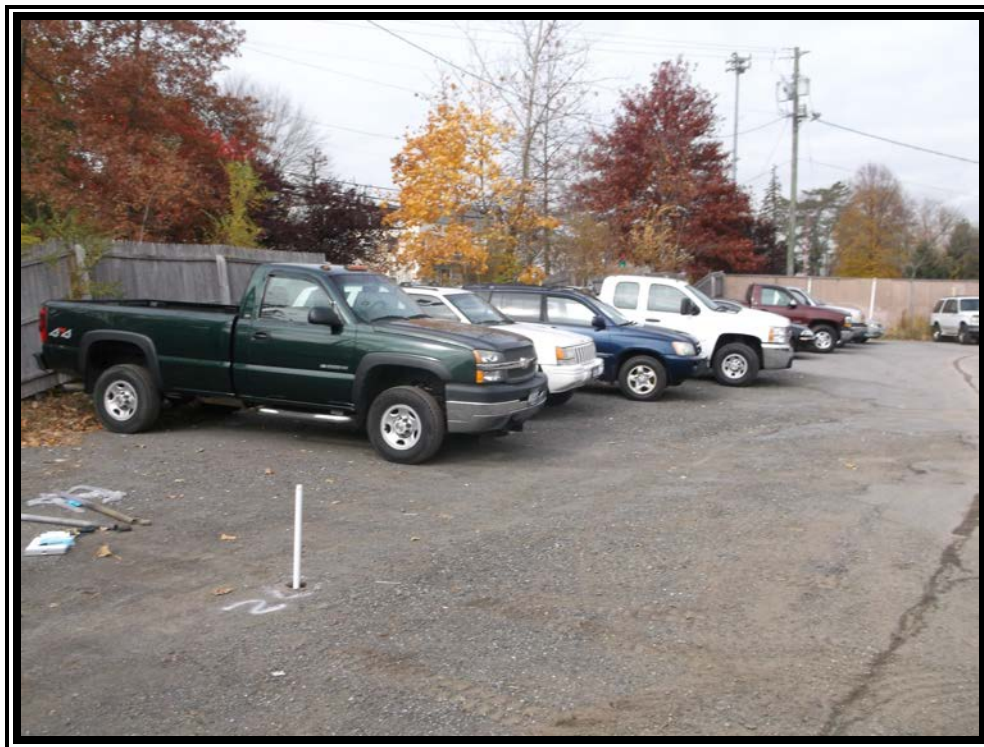
Photograph taken of the monitor well installed at the GB-7 location
